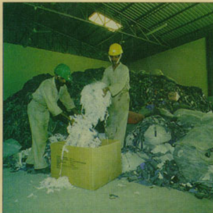
Waste cloth being recycled into paper at the Al Quoz factory.
